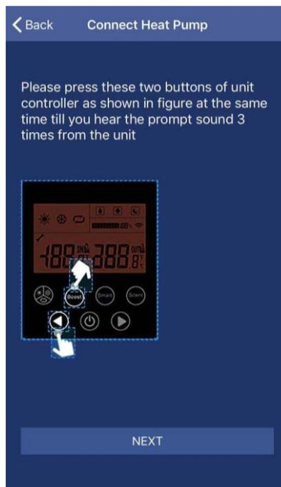
According to the introduction in the interface, please operate. After the heat pump unit setting, please press **Next**.
