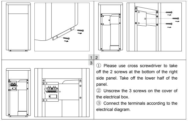
Note: For IPH20-35 model, please open the back panel for power connection. The operation is the same as above.
