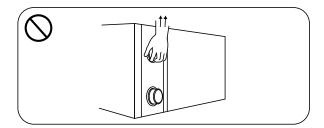
1.4.3. Don't put obstacles before the air inlet and outlet of the heat pump.
