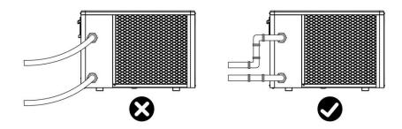
2.In order to guarantee the heating efficiency, the water pipe length should be  $\leq$ 10m between the pool and the heat pump.
