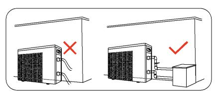
2.1.2. In order to guarantee the heating efficiency, the water pipe length should be ≤10m between the pool and the heat pump.
