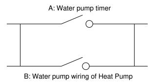
Note: The installer should connect A parallel with B (as above picture). To start the water pump, condition A or B is connected. To stop the water pump, both A and B should be disconnected.
