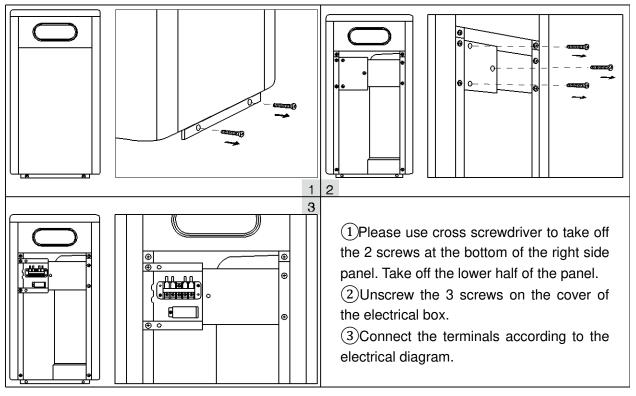
Note: For IPH28/35 model, please open the back panel for power connection. The operation is the same as above.
